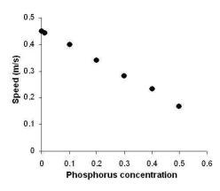
Figure 10. Speed of dendrite tip versus phosphorus concentration.
