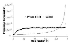
Figure 3. Comparison of phosphorus concentration, as evaluated via the Phase-Field Method, with Scheil's equation (Chalmers, 1964).
