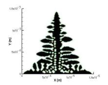
Figure 7. Dendrite simulated for a super-cooled domain.
