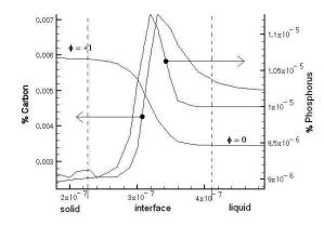
Figure 5. Carbon and phosphorus concentrations by region: solid ( $\phi = +1$ ), liquid ( $\phi = 0$ ), and interface ( $0 < \phi < +1$ ).
